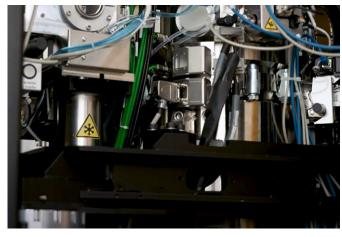
Inside a cryoElectron microscope at the University of Washington where studies of the molecular structures of coronavirus spike proteins takes place. The approach is a type of transmission electron microscopy for viewing samples at cryogenic temperatures. Credit: UW Medicine
