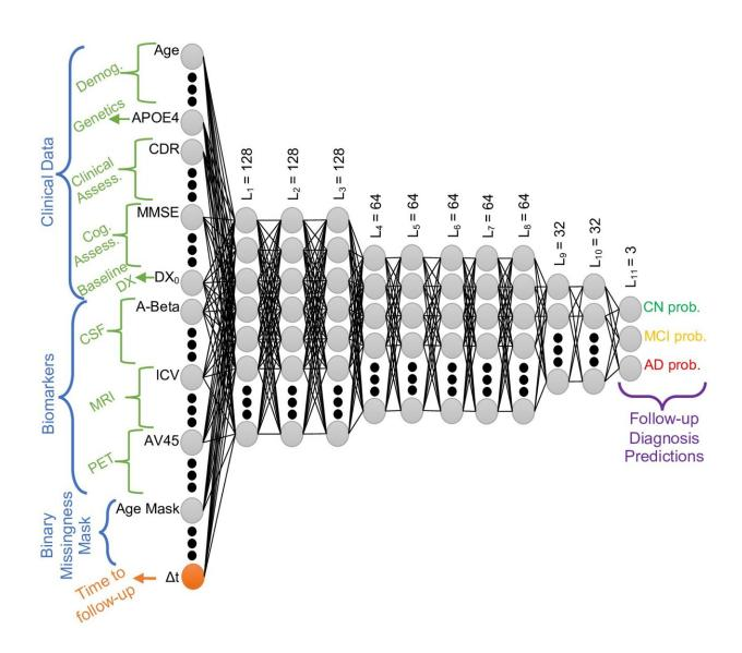
Feed-forward, fully-connected neural network architecture. Nonlinear models have rectified linear units (ReLU) between layers. Final layer implements a softmax. Ll: Number of neurons in layer l. Input features include following. Demog.:
