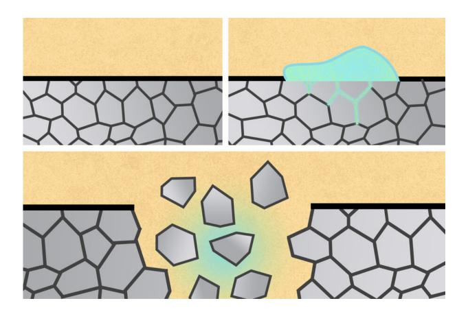
MIT engineers have shown that medical devices made from aluminum can be disintegrated within the body by exposing them to gallium-indium, a liquid metal that seeps into the boundaries between the grains of the metal. Credit: MIT News, based on figures courtesy of the researchers
