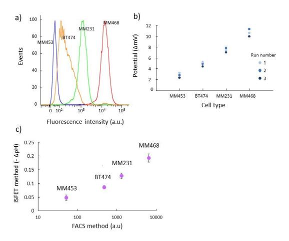
The results of membrane protein measurement using the cell-transistor correlate with the results of conventional fluorescence-activated cell sorting (FACS). Realization of an ultra-sensitive liquid biopsy platform based on semiconductor technology is expected. Credit: Department of Bioelectronics, TMDU
