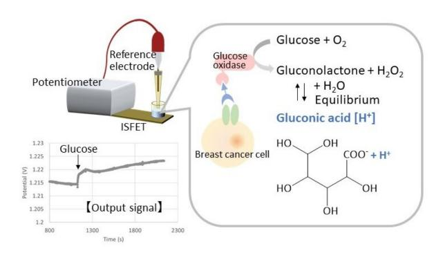
Ion-sensitive field effect transistors detect breast cancer cells expressing EGFR when bound by an antibody linked to a chemical reporter. Credit: Department of Bioelectronics, TMDU
