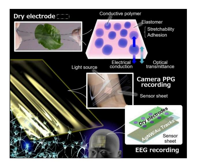
Image of dry-type bioelectrode and thin-film sensor sheet. Credit: Reprinted with permission from Advanced Materials Technologies, CC BY, Attribution 4.0 International (CC BY 4.0)
