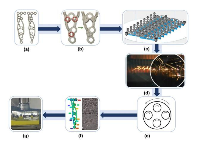
G-DfAM workflow for HTO plate fixations, a GD HTO plate conceptual designs, b design optimization of GD plate conceptual designs, c PBF-EB build preparation, d PBF-EB manufacture of Ti-6Al-4 V plates, e mass finishing, f optical surface inspection, g CNC machining of plate holes and threads. Credit: *Progress in Additive Manufacturing* (2022). DOI: 10.1007/s40964-022-00342-2
