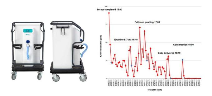
Ambient concentration of nitrous oxide in parts per million (ppm) with use of cracking technology, over the course of established labor, plotted against time. Picture of Mobile Destruction Unit (MDU) on the left of the chart (reproduced from the product literature with the manufacturer's permission). Credit: *Anaesthesia Reports* (2022). DOI: 10.1002/anr3.12182
