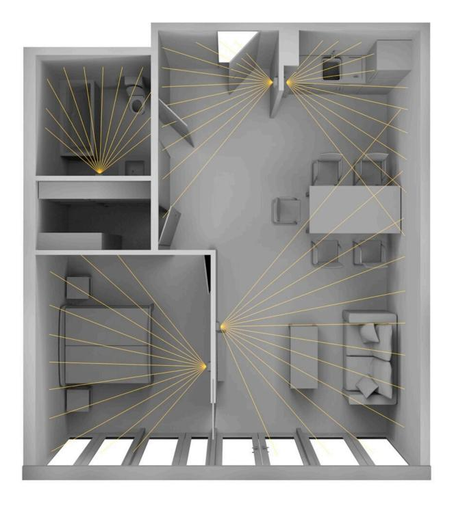
Exemplary apartment, highlighting the sensor system used in the study. Individual rooms are equipped with motion sensors, entrance and fridge doors are equipped with magnetic door sensors, and a bed sensor is placed beneath the mattress. Credit: NeuroTec/*Nature Scientific Reports*, Creative Commons Licence
