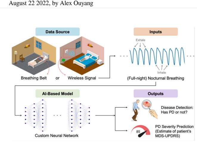
The system extracts nocturnal breathing signals either from a breathing belt worn by the subject, or from radio signals that bounce off their body while asleep. It processes the breathing signals using a neural network to infer whether the person has Parkinson's, and if they do, assesses the severity of their disease in accordance with the Movement Disorder Society Unified Parkinson's Disease Rating Scale. Credit: Image courtesy of the researchers.
