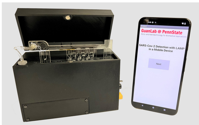
The SLIDE device analyzes saliva and could help make COVID-19 testing quicker and easier. Credit: Weihua Guan
