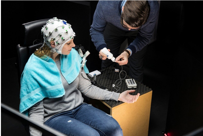
Mathias Vukelic preparing for an EEG measurement and using gel to improve the conductivity of the electrodes. Credit: AUDI AG
