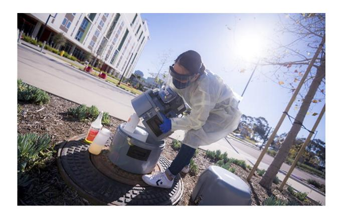
Auto-sampling robots at scores of sites on the UC San Diego campus collected wastewater samples, which were analyzed for levels of SARS-CoV-2 RNA by labs at UC San Diego, with further computational analysis conducted at Andersen's lab at Scripps Research. Credit: Erik Jepsen/UCPA
