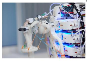
Humanoid bioreactor platform developed to provide engineered tendons with human-like mechanical stimulation. It consists of a robotic shoulder combined with a soft bioreactor chamber. The small chamber, positioned at the supraspinatus tendon location, contains human cells grown onto a biomimetic material and is filled with culture medium. Credit: Fisher Studios
