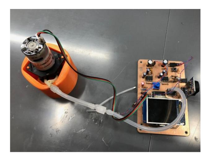
An early generation prototype of the tympanometer device that can modulate pressure, generate sound, and measure the reflected sound from the tympanic membrane. Credit: Duke University
