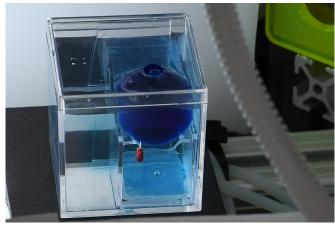
A simulation shows how a remote-controlled micro robot (with red body) could be used to puncture a cyst (represented by blue ball) in a child's brain.
