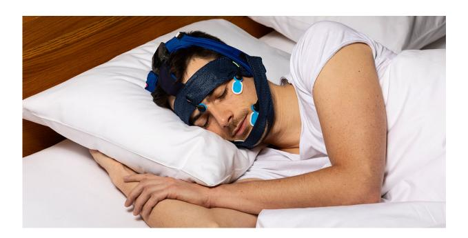
The SleepLoop system developed by ETH Zurich researchers emits a sound at the right time to amplify the slow brain waves. Credit: Sleeploop
