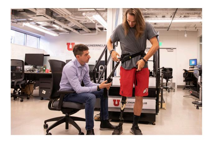
University of Utah mechanical engineering assistant professor Tommaso Lenzi (left), helps Alec McMorris put on an experimental exoskeleton that Lenzi has developed for lower-limb amputees. The lightweight powered exoskeleton allows users to walk with much less effort thanks to a series of motors, microprocessors and advanced algorithms. Credit: Dan Hixson/University of Utah College of Engineering
