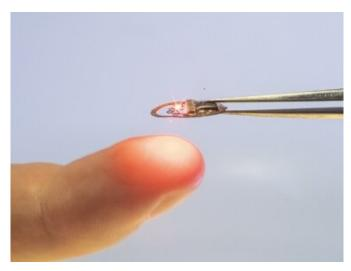
The wireless battery-free device, which is implanted just under the skin, is as thin as a sheet of paper and about half the diameter of a dime. Credit: College of Engineering
