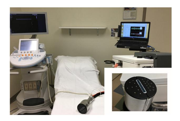
Quing Zhu's lab developed this handheld ultrasound-guided diffuse optical tomography system which consists of a 10-centimeter probe and a near-infrared system that takes data noninvasively from the breast from nine sources and 14 detectors in less than 4 seconds. Credit: Quing Zhu lab
