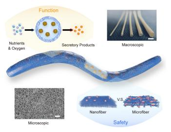
A schematic showing the structure and function of the NICE device, along with microscopic and macroscopic images. Credit: X. Wang et al., Science Translational Medicine (2021)
