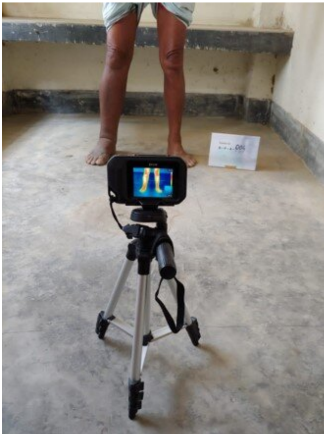
Camera set up for taking images of participants lower legs. Credit: Louise Kelly-Hope
