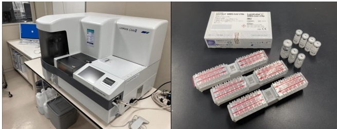
The Lumipulse G600II instrument (left) and the Lumipulse SARS-CoV-2 Ag kit (right), both manufactured by Fujirebio, which were used in this study for the quantification of SARS-CoV-2 in saliva samples. Credit: Shinichi Fujisawa
