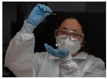
Due to their high-density grid layout, small size and their ability to conform to the hippocampal surface, the LLNLdeveloped micro-electrode arrays provided researchers with a critical "birds-eye-view" of how traveling waves moved and reversed over the surface of the
