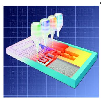
Using a 3D printer, the researchers fabricated a 3D version of a lateral flow test. The basis is a small block of porous polymer, in which 'inks' with specific properties are printed at precise locations. Credit: Ameloot Group
