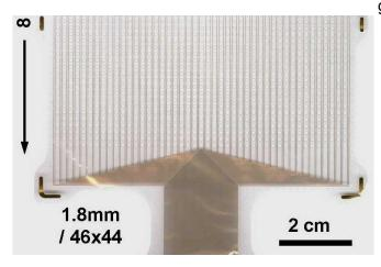
Image of one of a flexible mats of closely spaced sensors being developed at UC San Diego. These kinds of sensor grids are temporarily placed directly on the surface of the brain during some cancer and epilepsy surgeries. Credit: University of California - San Diego
