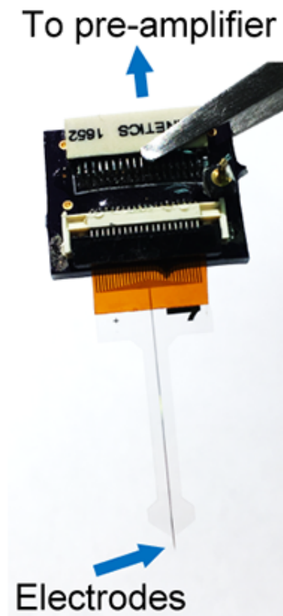
The neural implant connected to a custom printed circuit board. Credit: Nature Neuroscience
