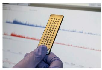
A target plate is used in a mass spectrometer. Proteins from the sample are ionized with a laser, then measured and analyzed to detect the SARS-CoV-2 virus. Credit: UC Davis Health
