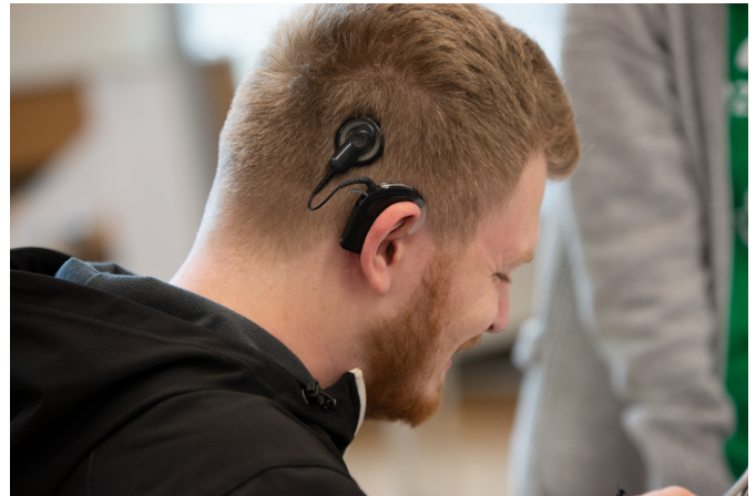
A young man with a cochlear implant. The cochlear implant is considered the most successful neuroprosthesis, providing speech understanding in quiet background to more than 700,000 users worldwide. Credit: Karin Tilch/Deutsches Primatenzentrum
