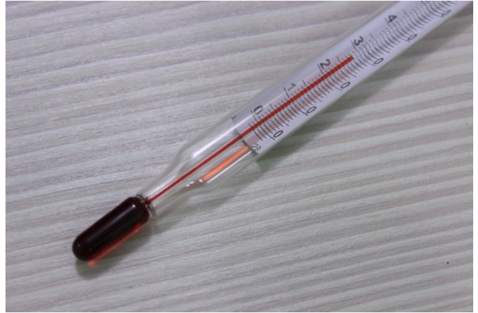
A modern liquid thermometer, which works by the change in volume of a thermometric fluid, mostly coloured alcohol. Credit: MZinchenko/Shutterstock.com
