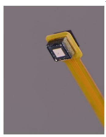
A block module of a 3-?m-diameter and 400-?m-length needle-electrode (frontside block, 1 × 1 mm2) is stacked on an amplifier module (backside block) via a flexible interposer. Credit: Toyohashi University of Technology.
