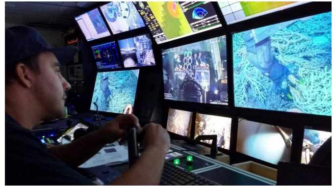
ROV pilot Adam Whetmore flies the submersible SuBastian onboard the R/V Falkor to collect a coral sample with its robotic arm, at the direction of the science team. Credit: Schmidt Ocean Institute
