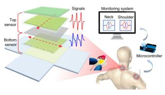
Schematic illustration of the system to prevent joint disorders. The signals produced from the attached sensors are transmitted to an intelligent terminal through a microcontroller. The multilayer sensor consists of a cross-shaped substrate, a square top sensor and a square bottom sensor. Credit: Dr. Zhengbao YANG from the City University of Hong Kong
