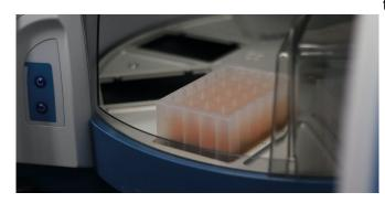
Sewage samples mixed with magnetic beads and loaded onto the liquid-handling robot for viral concentration. Credit: C. H. Sheikhzadeh @ HOMA Photographic Art
