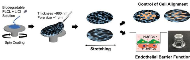
Overall schematic illustration of the fabrication of EPUM using PLCL using a VIPS process during spin-coating. The fabricated membrane was transferred to a 12-well insert for cell co-culture to mimic an endothelial barrier model. Credit: Korea Institute of Science and Technology(KIST)
