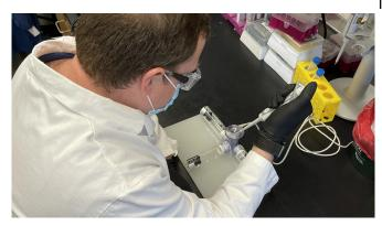
Researcher Daryll Vanover works with the nebulizer he adapted to test a new mRNA-based treatment for flu and Covid-19. The team used mRNA technology to code for a protein called Cas13a that destroys parts of the RNA genetic code that viruses use to replicate in cells in the lungs. It was developed by researchers in Philip Santangelo's lab in the Wallace H. Coulter Department of Biomedical Engineering. Credit: Georgia Institute of Technology
