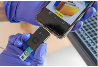
Programmed magnetic nanobeads paired with an off-theshelf cellphone and plug-in diagnostic tool can diagnose COVID-19 in 55 minutes or less, according to Rice University engineers. Credit: Jeff Fitlow/Rice University
