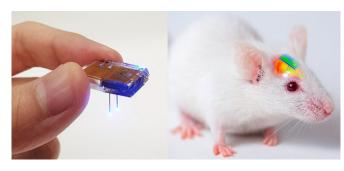
Optical image of a wirelessly rechargeable, soft optoelectronic system held with fingers. The device is emitting blue light from its bilateral probes. Credit: The Korea Advanced Institute of Science and Technology (KAIST)
