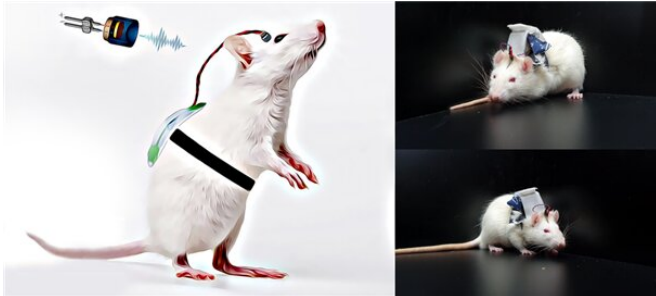
Photographs of animal model using the developed wireless wearable brain stimulation system. Credit: Korea Institute of Science and Technology (KIST)
