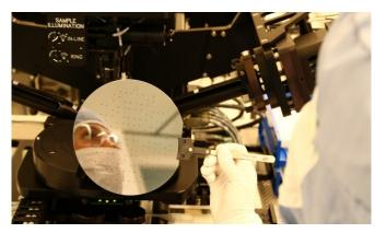
Researcher and author Elizaveta Vereshchagina in the laboratory. Microfluidics technology has a variety of applications, including DNA analysis and organ-on-achip. The photo shows a 6-inch silicon wafer during processing in cleanroom. The dots are inlets to and outlets from the microfluidic channel. Credit: Norwegian University of Science and Technology
