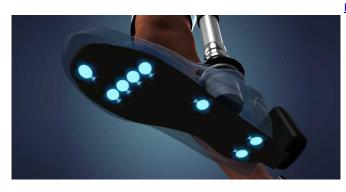
Signals from tactile sensors under the sole of the prosthetic foot and from angle sensors in the electronic prosthetic knee joint are passed on to the nervous system. Credit: ETH Zurich
