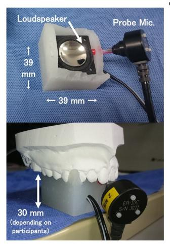
Excitation setup for measuring transmission characteristics. A loudspeaker was embedded in an enclosure fitted to the hard palate to make a quasi-static sound field in the OC. The probe microphone was placed in the sound field for measuring the response signal. Credit: Masashi Unoki from Japan Advanced Institute of Science and Technology
