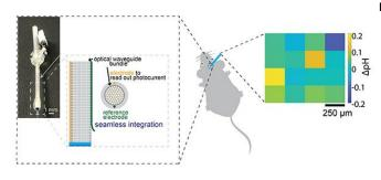
The multiplexed pH probe with a light-addressable potentiometric sensor and a schematic diagram of the multimodal fiber. The implantable device can acquire real time multi-site acquisition to detect pH levels in vivo. Credit: Tohoku University
