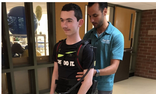
A study participant undergoing gait training in the EksoGT administered by a licensed physical therapist. Credit: Kessler Foundation
