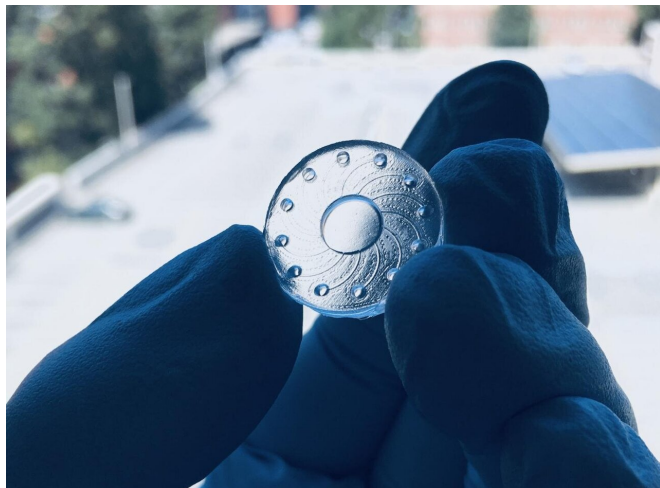
Enlarged prototype of biosensor lens with reservoirs. Credit: Khademhosseini Lab
