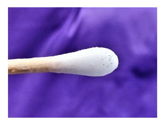
A theragripper is about the size of a speck of dust. This swab contains dozens of the tiny devices. Credit: Johns Hopkins University.
