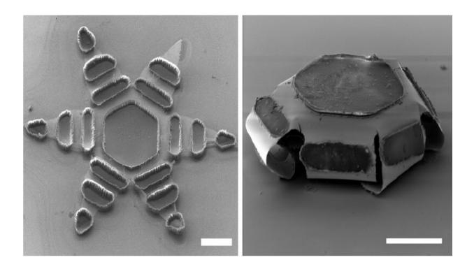
When an open theragripper, left, is exposed to internal body temperatures, it closes on the instestinal wall. In the gripper's center is a space for a small dose of a drug. Credit: Johns Hopkins University
