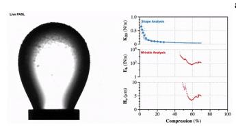
Researchers used pendant drop elastometry to compress and expand the biofilm that the PASL cells formed. Credit: Tagbo Niepa / University of Pittsburgh Swanson School of Engineering
