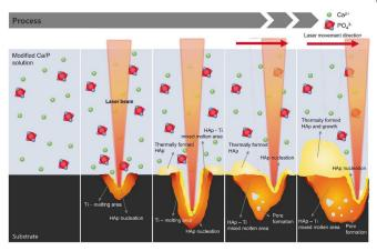
Schematic diagram of the laser-induced single-step coating induced hydroxyapatite synthesis, HAp-substrate mixed molten layer, and HAp coating layer formation process. In the figure, the green and red circles indicate "Ca2+", and "PO43." ion, respectively. Credit: Korea Institue of Science and Technology(KIST)
