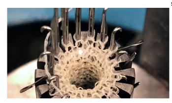
Researchers used a circular knitting machine to make a prototype of a replacement for a coronary artery. Credit: Fan Zhang.
