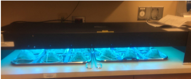
Multiple N95s under UV-C light. Credit: Henry Ford Health System / University of Michigan
