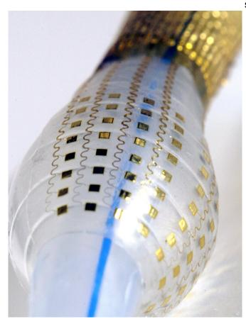
Seen here, a conformal array of electrodes affixed to an inflated balloon catheter. Credit: John Rogers/Northwestern University
